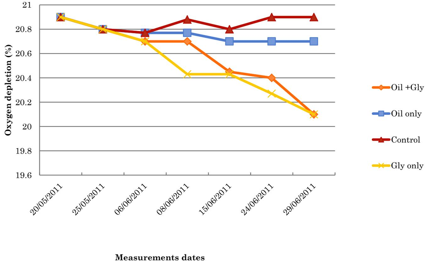
Fig. 3: O<sub>2</sub> depletion trend from the rigs: 20/05/11 to 25/06/11 represent background studies. Contaminants were added on 06/06/11 followed by weekly contaminant addition. Error bars represent the mean  $\pm$  S.E. of three replicates (triplicate measurements were virtually the same in many cases thus, the error bars are not observable)
