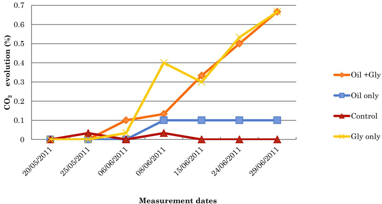
Fig. 2: CO<sub>2</sub> evolution trend from the rigs: 20/05/11 to 25/06/11 represent background studies. Contaminants were added on 06/06/11 followed by weekly contaminant addition. Error bars represent the mean  $\pm$  S.E. of three replicates (triplicate measurements were virtually the same in many cases thus, the error bars are not observable)
